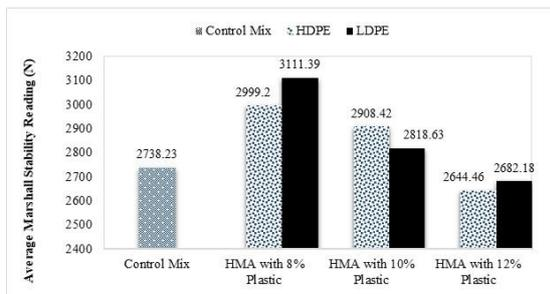
Figure 2. Average Marshall stability of hot mix asphalt control and modified mix.
