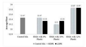
**Figure 3.** Average values of Marshall flow of hot mix asphalt control and modified mix.
