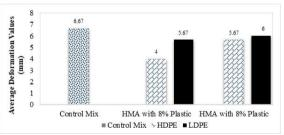
**Figure 4.** Deformation of hot mix asphalt with and without plastic wastes.
