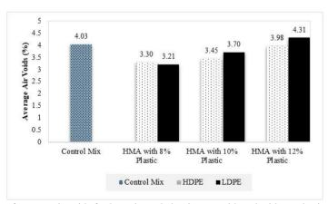
Figure 1. Average values of percent air voids for hot mix asphalt mixtures with and without plastic content.
