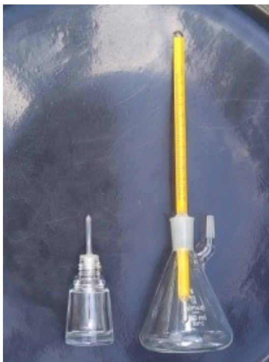
Figure 4. Improvised pycnometer (left) and standard pycnometer (right).
