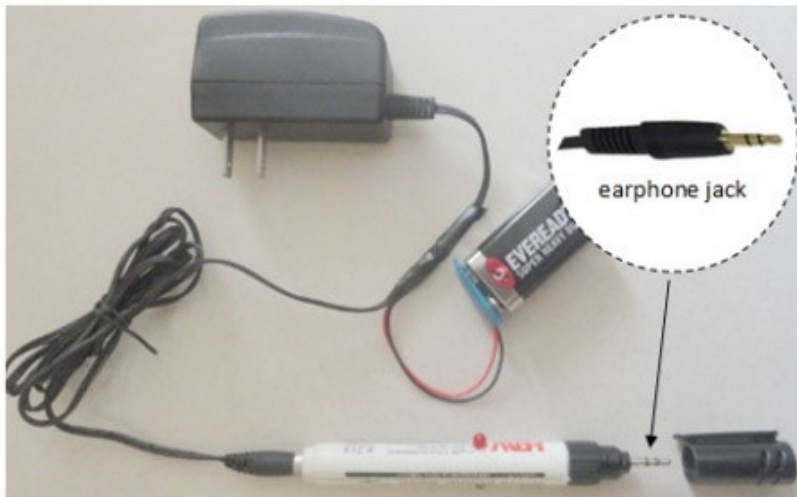
Figure 3. Circuit diagram for modified conductivity meter (top) and fabricated conductivity tester (bottom).
