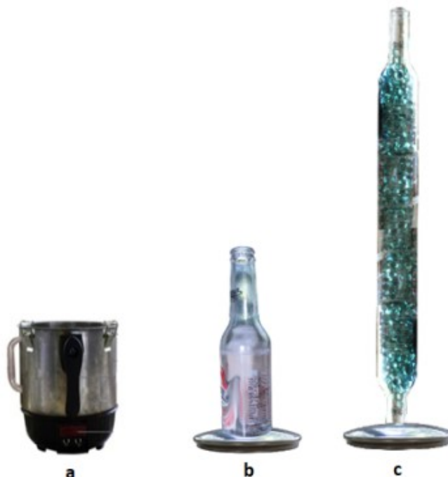
Figure 5. Electrothermal cup (a) and distilling lid for simple/steam distillation (b) and fractional distillation (c).
