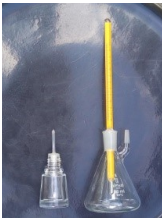
Figure 4. Improvised pycnometer (left) and standard pycnometer (right).
